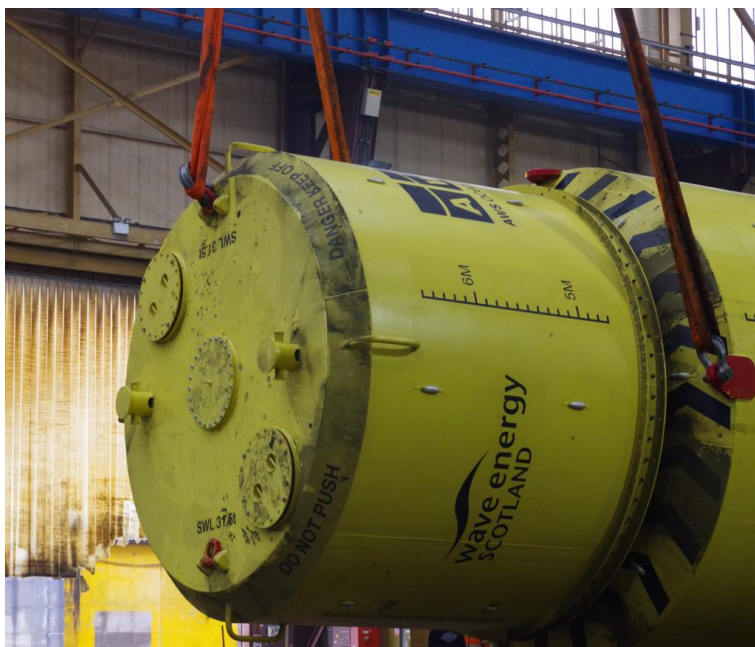
Figure 2- Shows position of side hatch (1200mm x 600mm) for man access. No man access planned whilst at sea.
