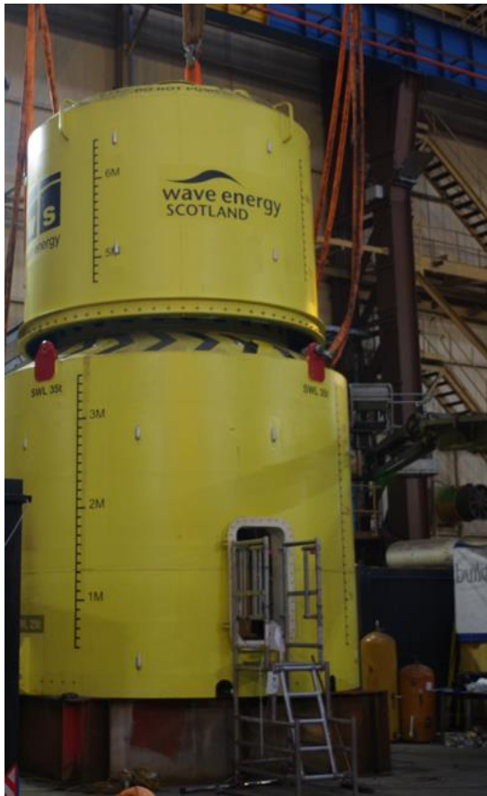
Figure 2- Shows position of side hatch (1200mm x 600mm) for man access. No man access planned whilst at sea.
