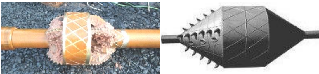
Figure 31. Typical fly-cutter hole opener (left) and Barrel Reamer (right).
