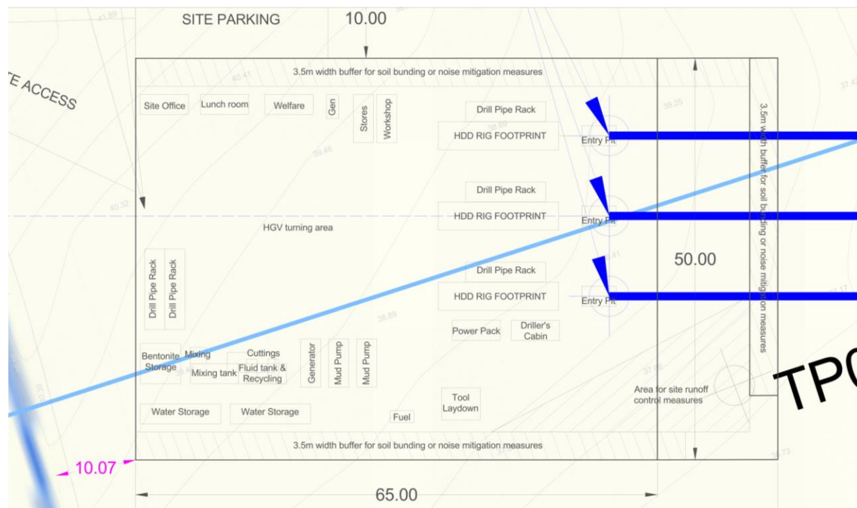
Figure 16. Detail of HDD site showing indicative positioning of equipment for Southern Design 5.
