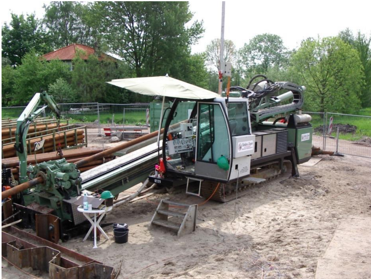
Figure 28. Example a midi sized HDD rig. The rig is anchored with sheet piling in this case.
