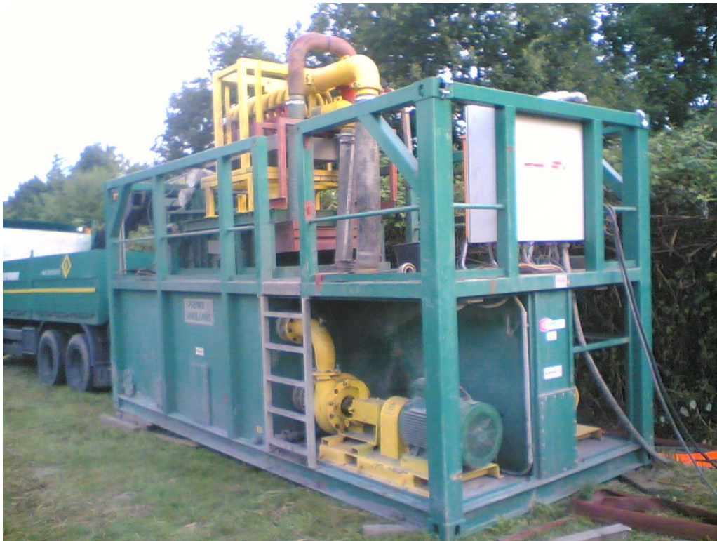
Figure 30. Drilling Fluid (“Mud”) Recycling Unit for midi sized HD rig.
