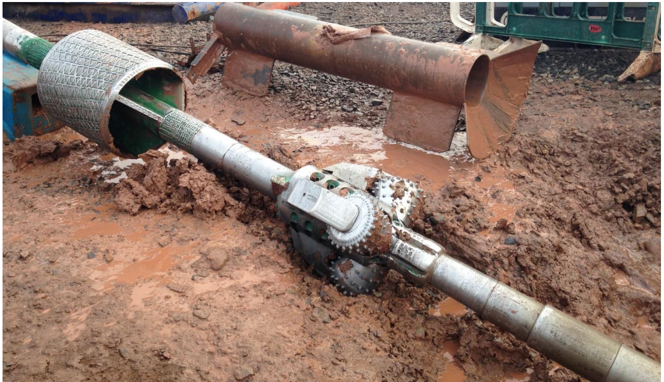
Figure 20. Typical forward reaming assembly for rock containing a TCI rock hole opener (right) with rear centraliser (left).
