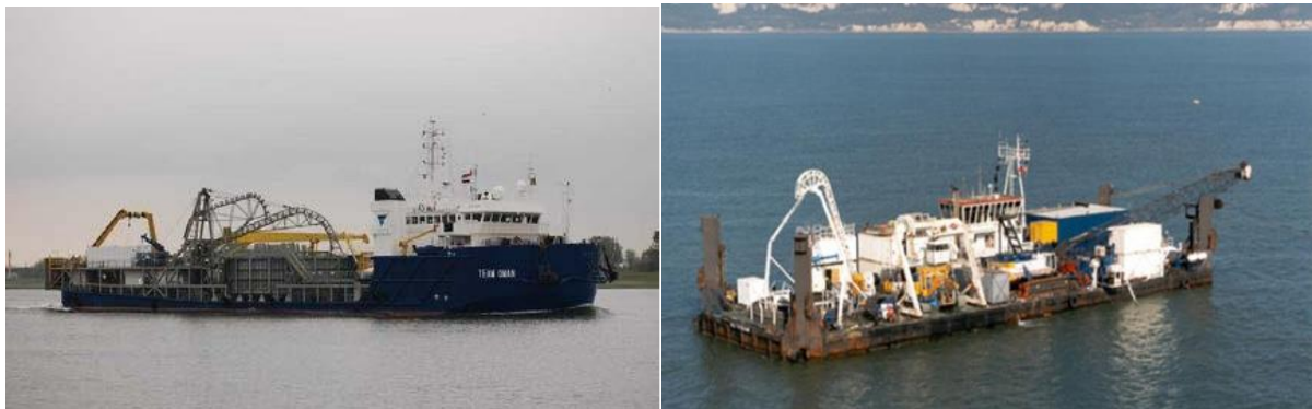
Figure 3: Representative Cable Laying Vessel and Cable Lay Barge
