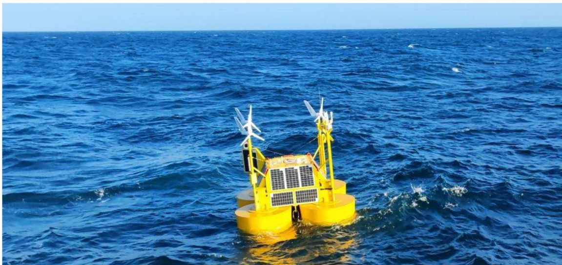
Plate 6.1: Floating LiDAR Positioned within the Bellrock WFDA
