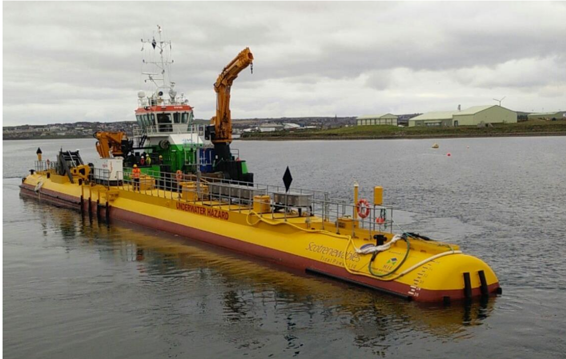
Figure 17: Multi-functional work vessels such as multi-cats are capable of precise movements of platforms in close-quarters and have capacity to tow turbines alongside owing to low well fendered free-board.
