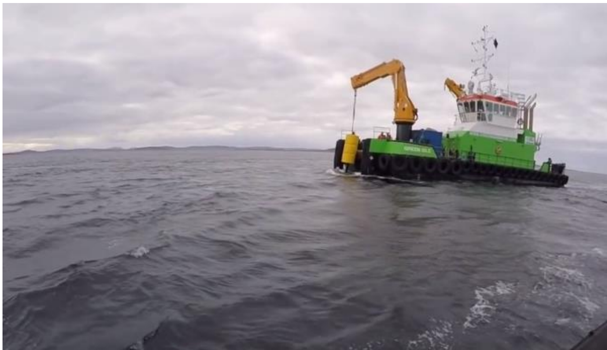
Figure 18: Installation vessel must have capacity for working with 2t buoys in tidal stream during pre-connection operations.
