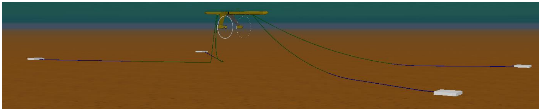
Figure 4 Orbital O2.4 mooring system operating in tide (green lines are 95mm Studlink chain, blue lines are 115mm studlink)
