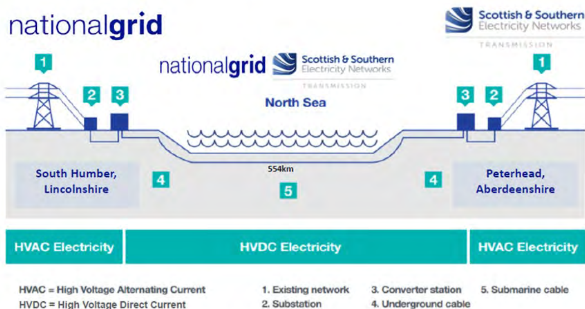
Figure 1-1 : Main infrastructure components of EGL 3
