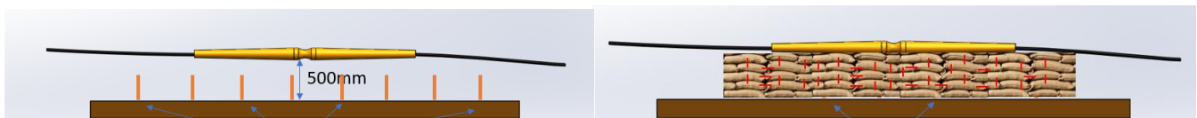
Drilled pins for grout bag holding
