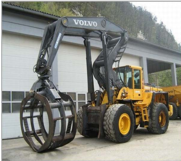
Fig 1 : Volvo L180H HL – is a bespoke design for log handling.
