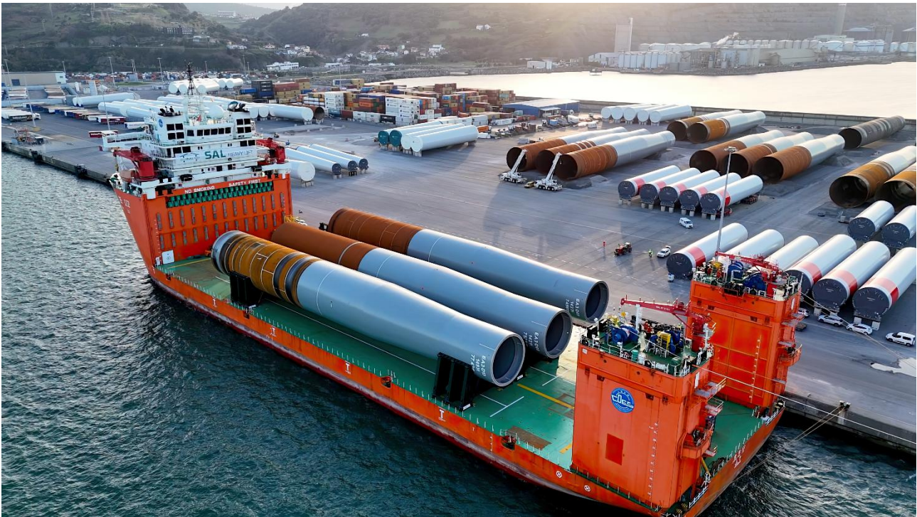
Plate 3.3 WTG Monopile Foundations from SPR's East Anglia THREE Offshore Windfarm Project
