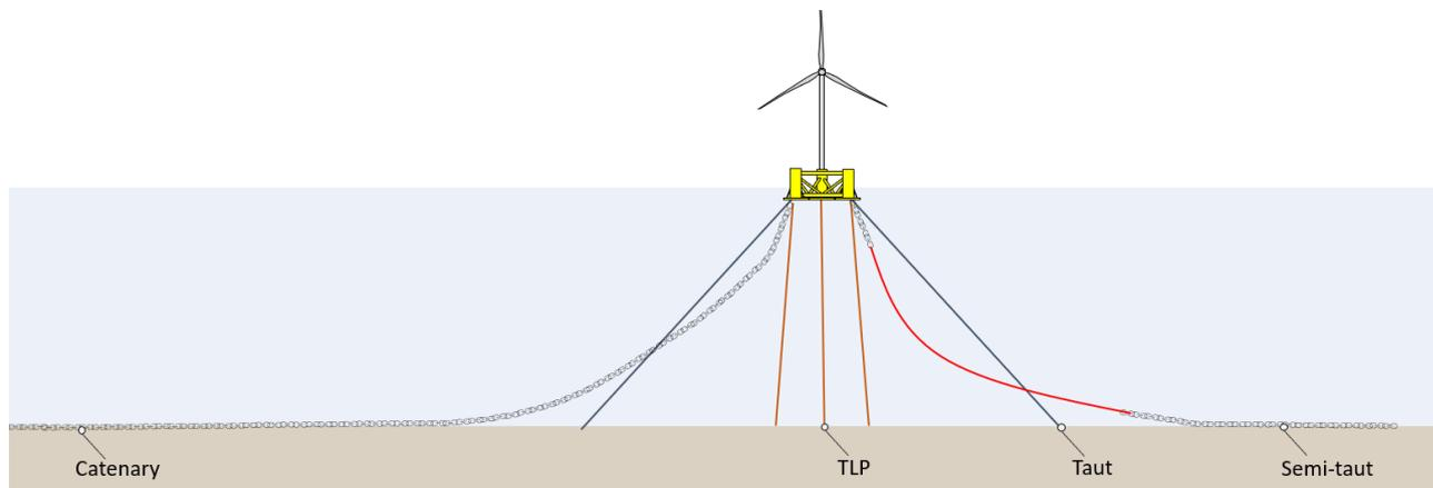
Figure 5.5 Illustration of potential mooring system configurations
