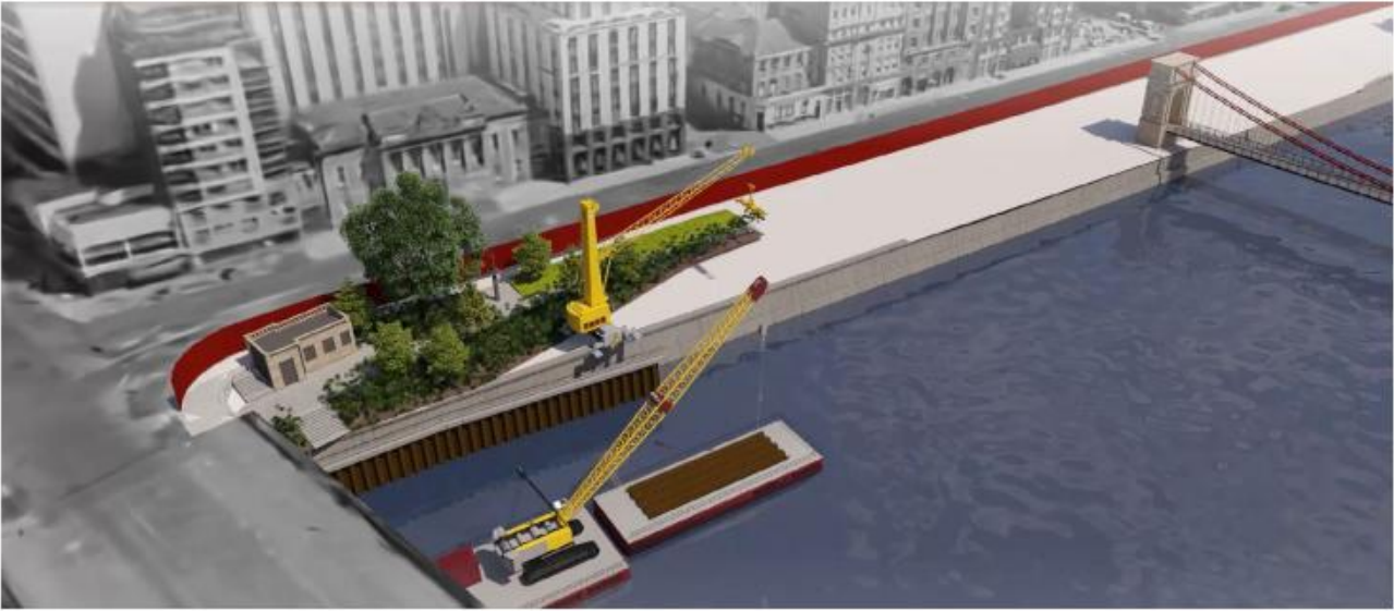
Figure 7 – 3D model of sheet pile installation
