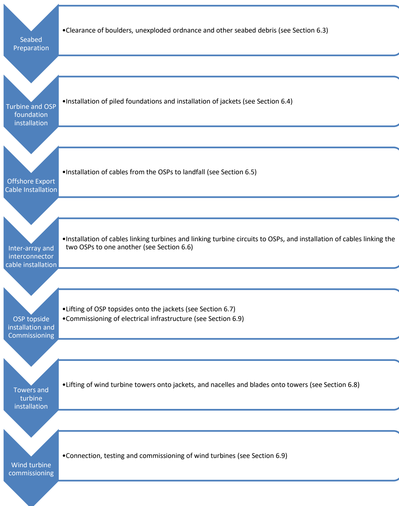
Figure 6-1: Overview of the Wind Farm and O&TW installation process
