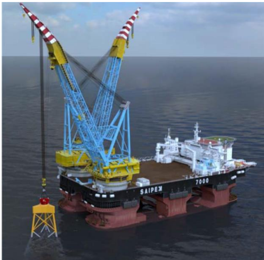
Figure 6-6: Deployment of the jacket from the SSCV
