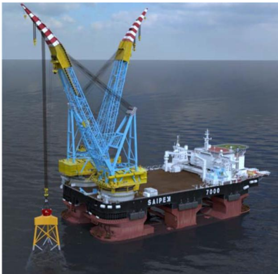
Figure 6-6: Deployment of the jacket from the SSCV
