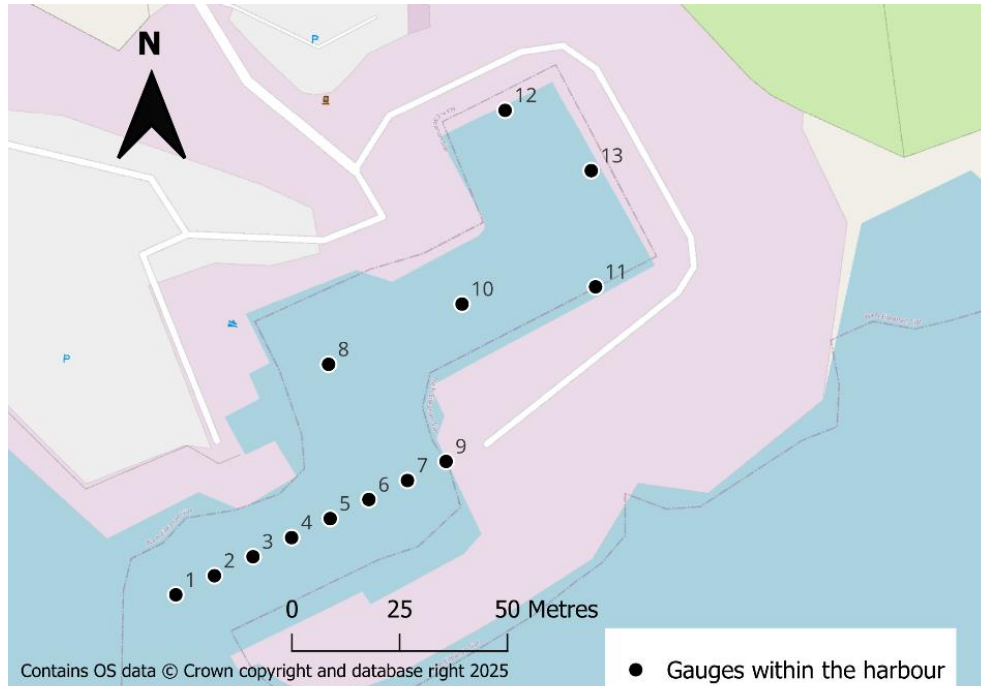
Figure 2-5 Schematic of the computational domain, representing the location of the gauges within the harbour.
