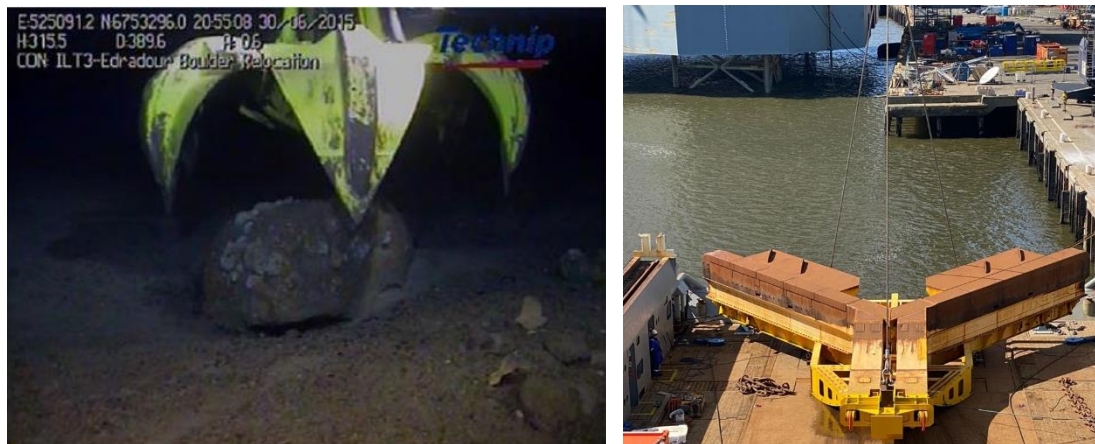
Figure 4-1: Example of a boulder grab system (left) and scar plough (right).
