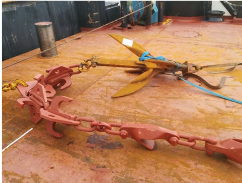
Figure 4-12: Example of a typical PLGR train on board the vessel.
