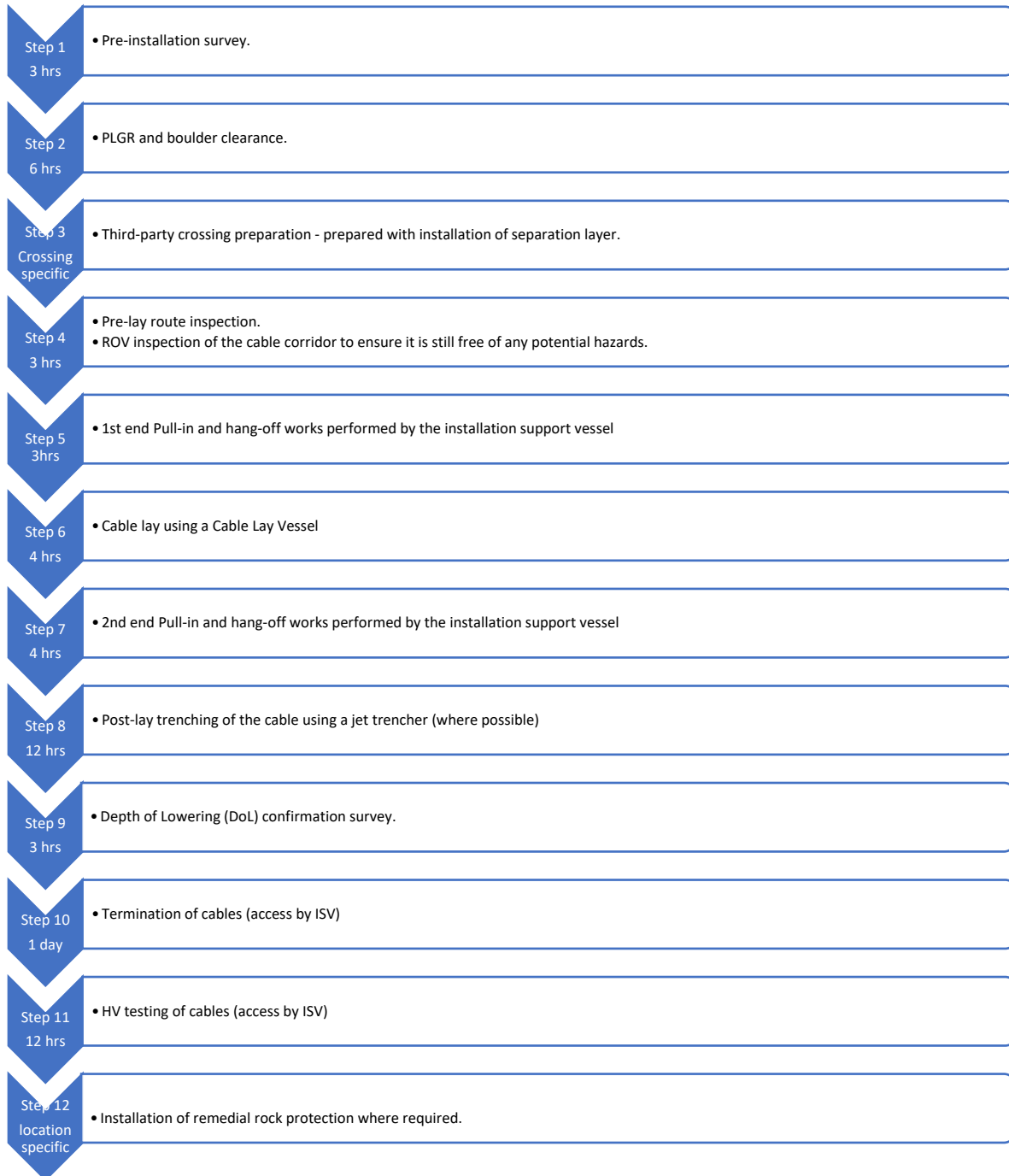
Figure 4-111: Overview of the inter-array and OSP inter-connector installation
