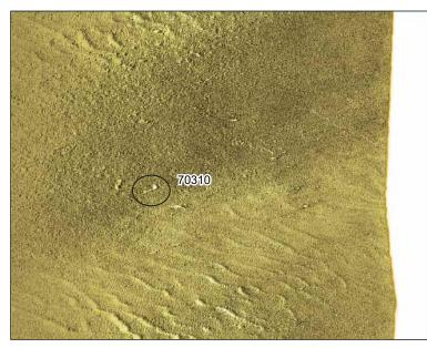
Sidescan sonar image of debris **70310**, measuring 7.8 x 0.7 x 0.1 m
