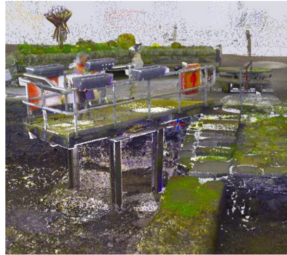
Fig 2.1.3 Laser survey of site showing existing viewing platform © Richard Ayling
