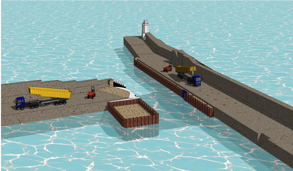
Stage 4 Works – Completion of pile driving and placement of backfill
