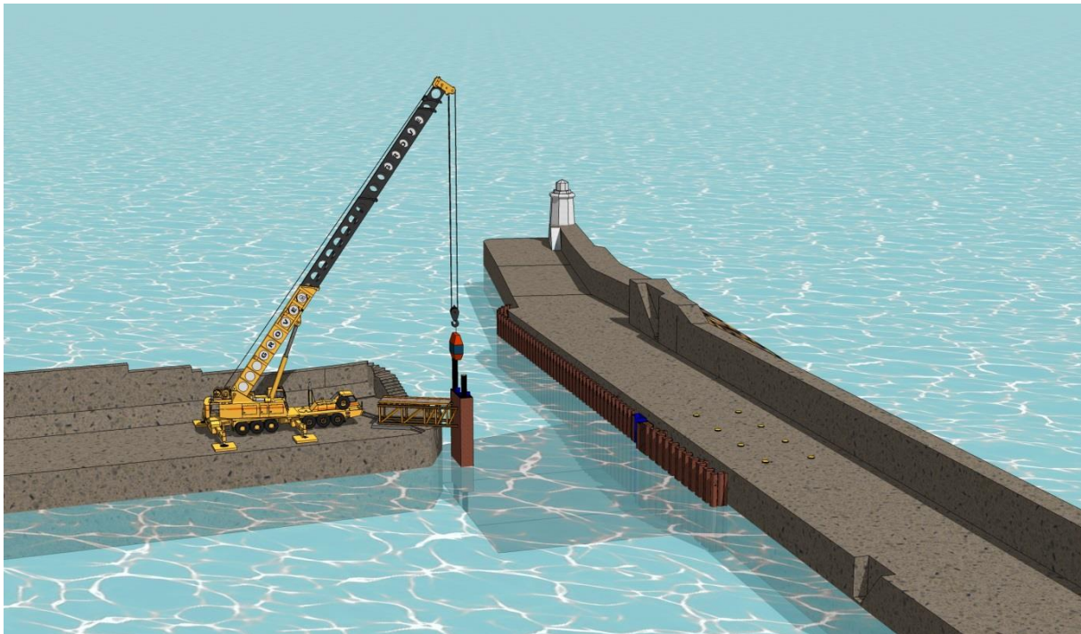
Stage 2 Works – Driving of Guide Frame to North Pier
