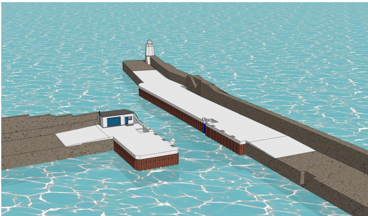
Stage 5 Works – Placement of Surface Slabs and Construction of Control Building
