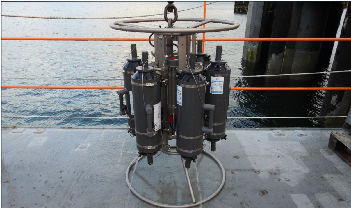
Figure 9 Rosette sampler equipped with Niskin bottles and CTD sensors.
