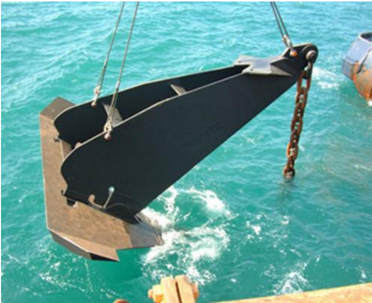
Figure 4-9 Example of a Stevpris Mk5 drag anchor
