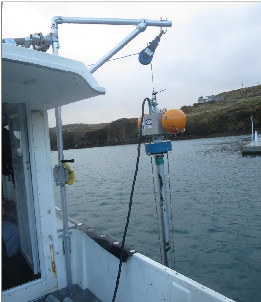
FIGURE 4 - VIBROCORE DEPLOYED ON REMOTE SENSOR
