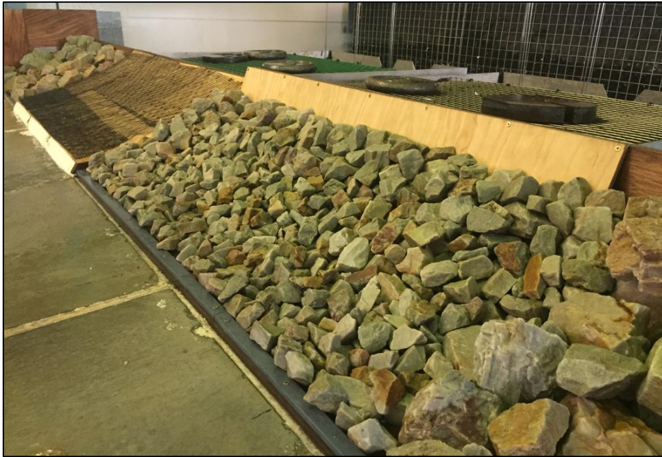
Figure 2.3: Photograph of the 50th Scale Existing Breakwater Model
