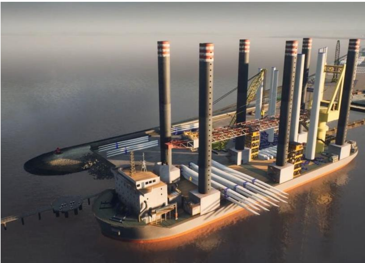
Plate 3-4 Example loading of offshore renewables vessel when berthed
