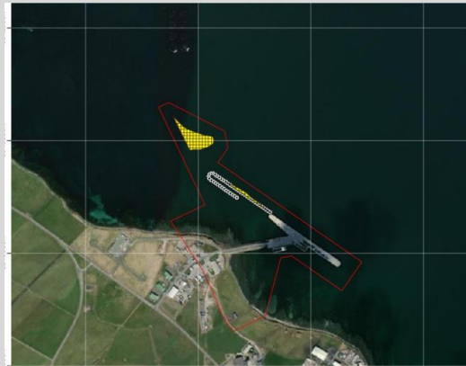
Above overview of assumed piling/blasting locations and approximate areas to be dredged
