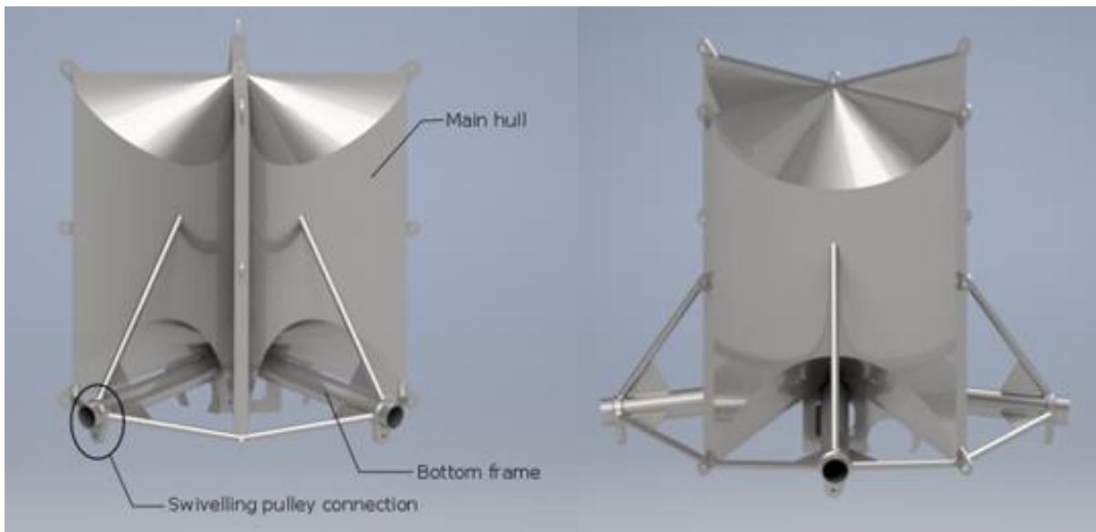
Figure 7: Front and side view of the Laminaria WEC (drawing)
