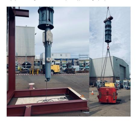
• Quayside testing that followed the same process as the workshop testing but with the test rig and receptacle cantilevered off a vessel, and the plug moored to the seabed via chains and clump weight anchors.
