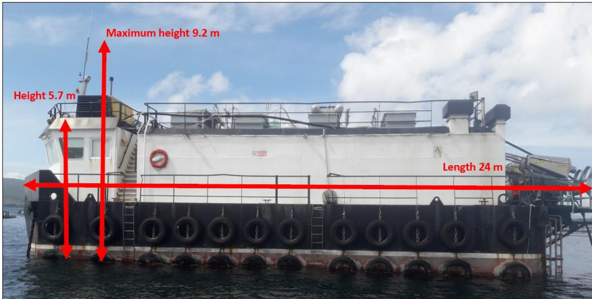
Figure 10. EXISTING & PROPOSED: Feed Barge Option 2. Approved by 18/04534/PNO Profile of the 200T steel barge showing height above seawater, maximum height, and length
