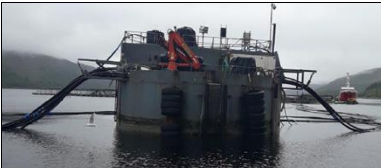
Figure 9. EXISTING & PROPOSED: Feed Barge Option 1 - Installed & Licenced by FFR/HLD/011 Profile of the Circular Concrete Auto-Feed Pontoon (C-CAP) (10m diameter, Height, 3.5-6m)
