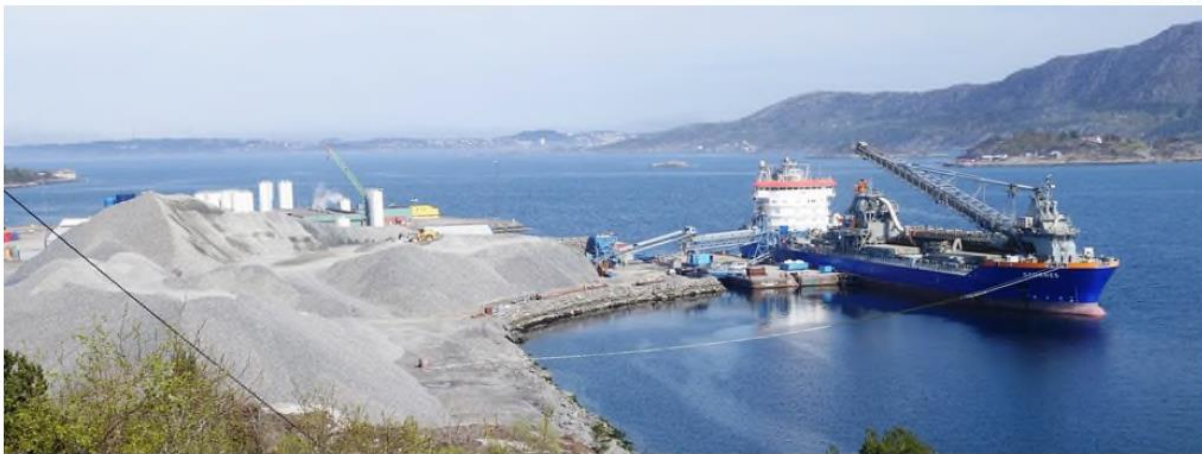
Figure 8 typical example of a FFPV loading rock at a quarry
