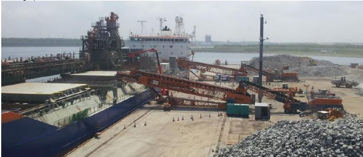
Figure 9 loading a FFPV via conveyor belts
