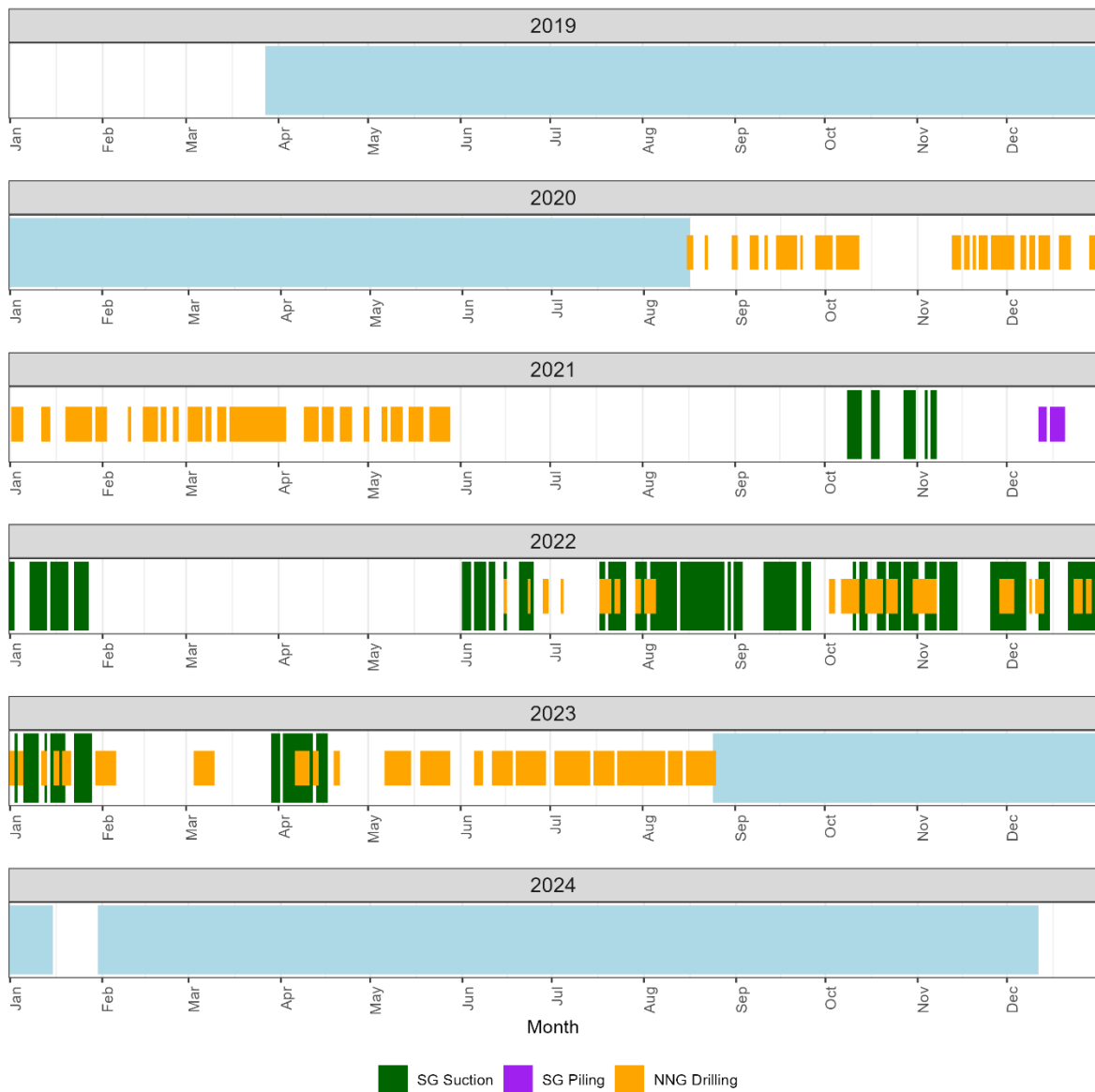
Figure 5-4. Construction activities at the two wind farms: suction and piling at Seagreen (green and purple) and drilling at NnG (orange). Light blue shades depict pre- and post-construction periods.
