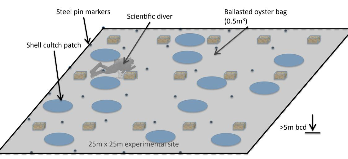
Schematic shows one of the two experimental sites with 15 bags deployed and cultch patches randomly in half the 5 x 5m plots. Bags recovered at 6 month intervals over 18 months. All recovered by end.
