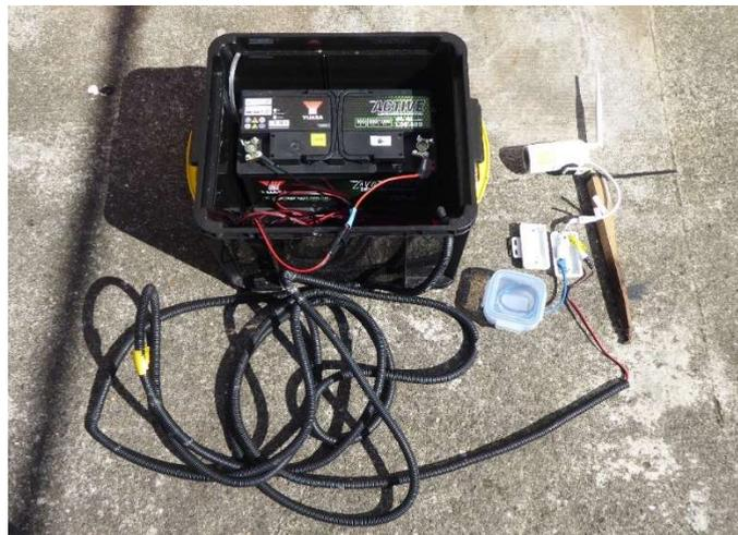
*Fig. 9. Motion detector camera set up. Upper photo shows camera on short wooden post trained on a puffin burrow, with battery placed in waterproof black box. Lower photo shows full set up with contents of box visible.*
