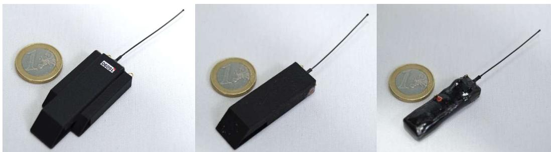
*Fig 1: Three Pathtrack devices used in the project: 11g logger used on guillemots (left panel), 8.2g logger used on razorbills and puffins (middle panel), and 4.1g used on puffins and kittiwakes (right panel). €1 coin provided for scale. See text for full details.*
