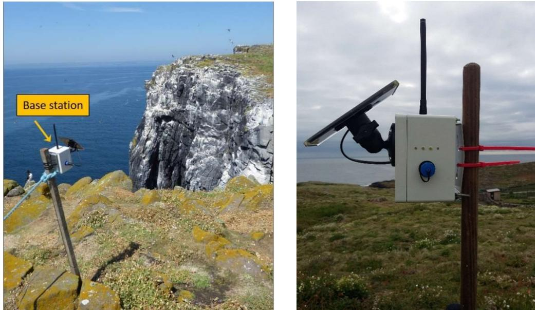
*Fig. 5: GPS tracking set up for remote download loggers. Left panel: base station positioned in proximity to breeding ledges; right panel: close-up of base station.*
