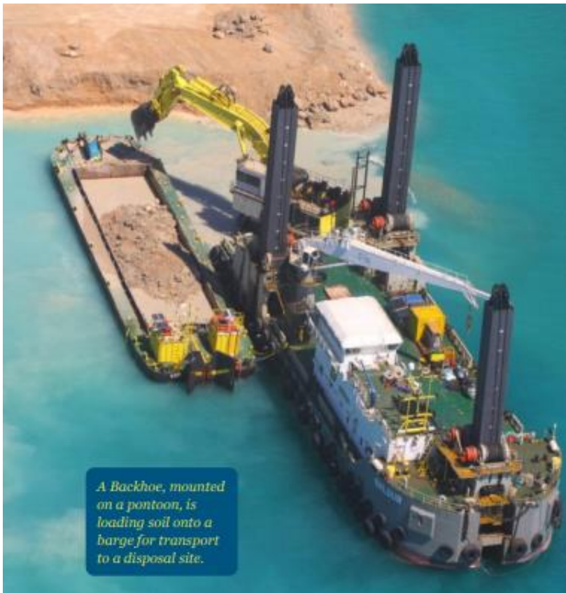
Figure 2.2: Backhoe Dredger Example
