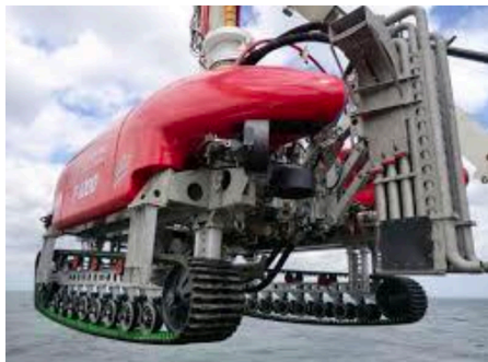
Water jetting seabed trencher (above)
