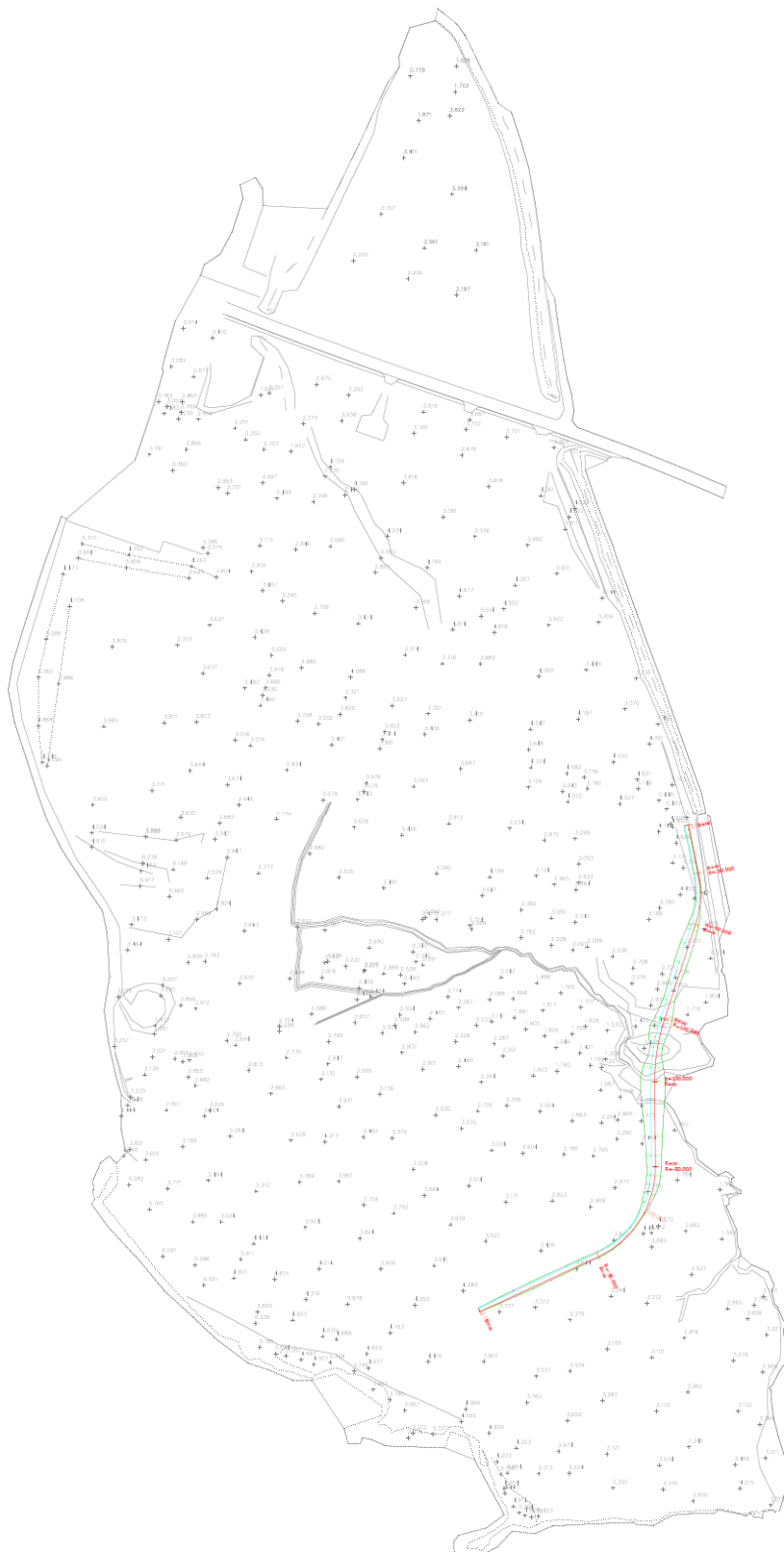
3.2.10 Figure 3-6 shows the 2D design model of the sites existing ground levels and the general arrangement for the Linclate Flood Protection Bund.
