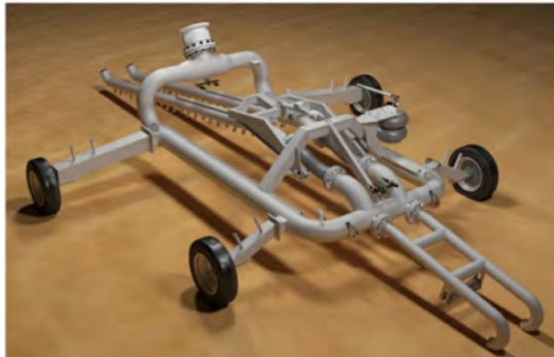
Figure 2-14 Typical diver assisted jet burial tool
