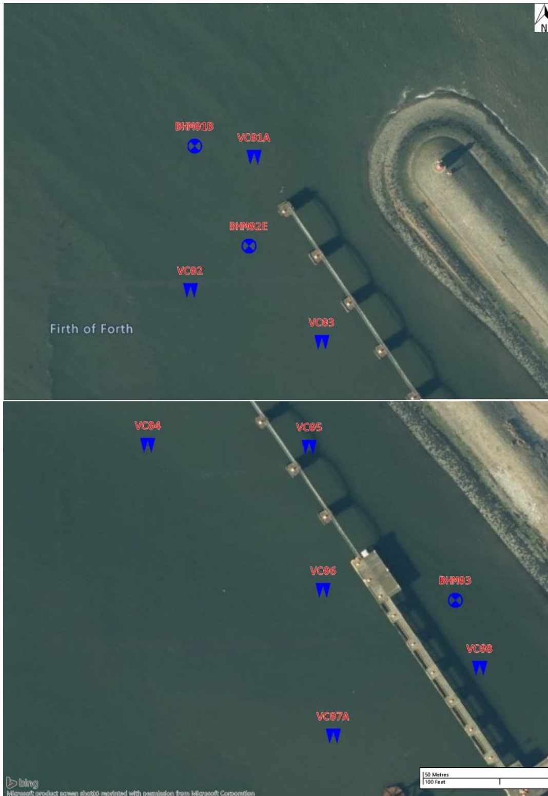
Figure 4.4 Location of boreholes and vibrocore samples undertaken in 2021 (Dunelm, 2022a)
