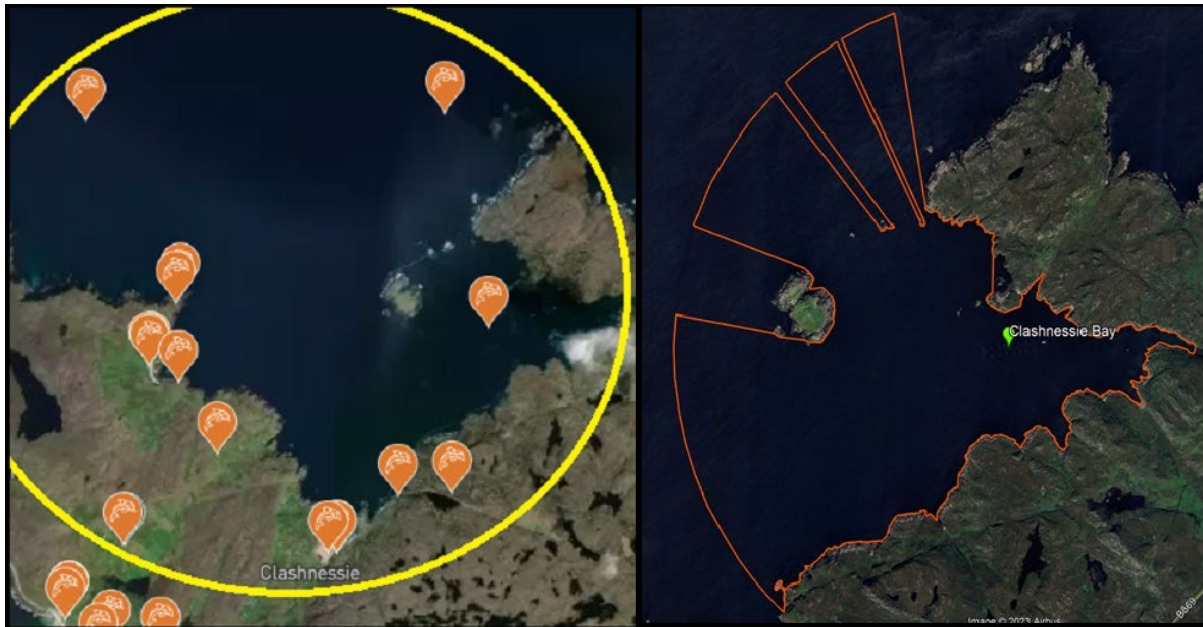
Image 1: Area from which sightings on HWDTT were counted (Inside the yellow circle) on the left. On the right is the disturbance threshold radiance of an Ace Aquatech RT1 system based at the Loch Duart Clashnessie site operating at its highest possible power level.
