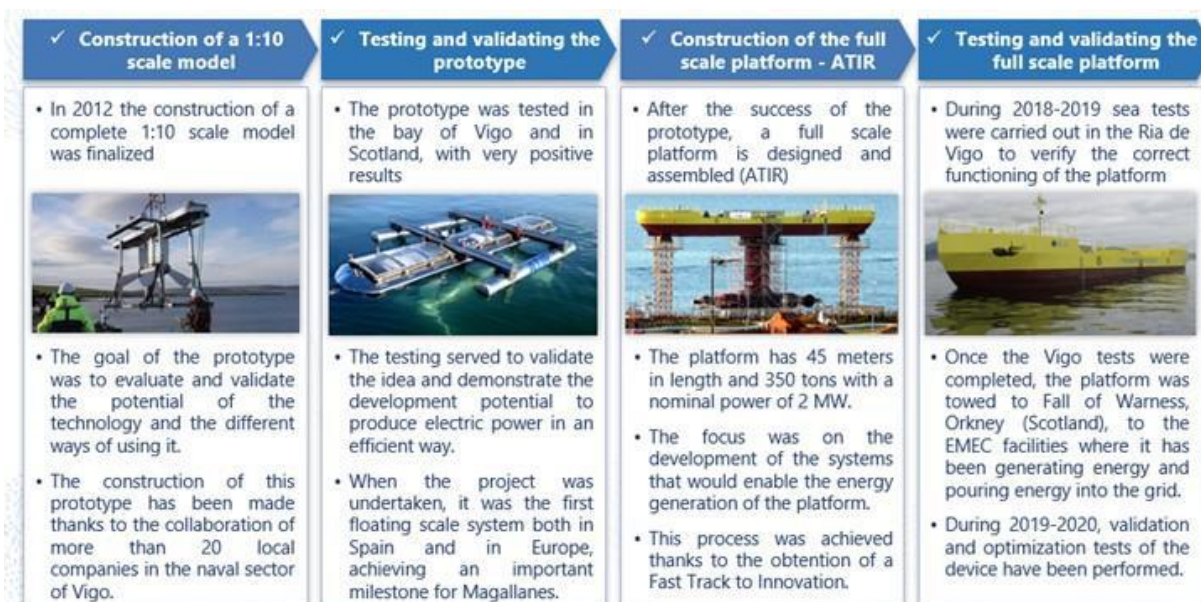
Figure 1| Evolution of the Magallanes Tidal Energy Technology
