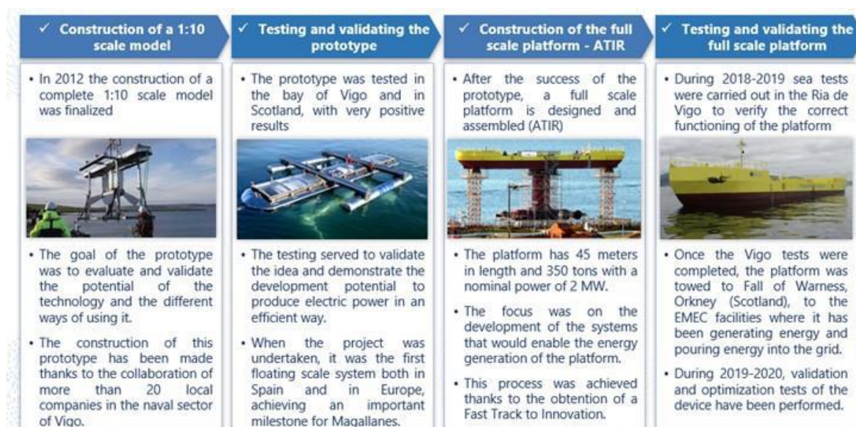
Figure 1| Evolution of the Magallanes Tidal Energy Technology
