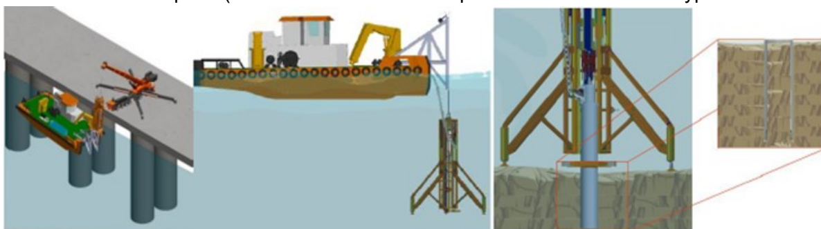
Figure 17| Images showing drill rig loadout, deployment to seabed and drilling
