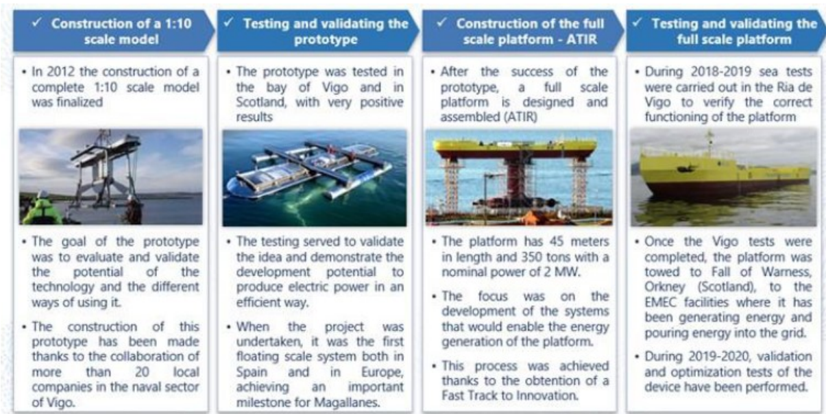
Figure 1| Evolution of the Magallanes Tidal Energy Technology
