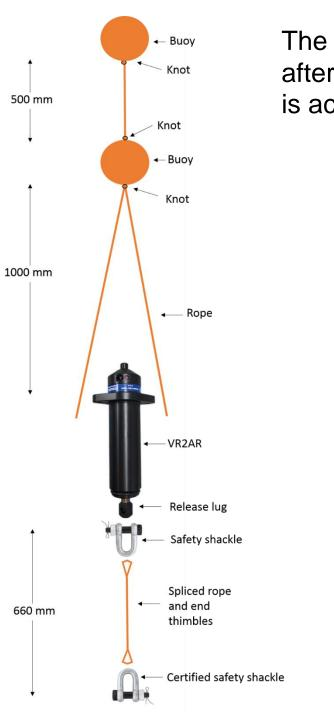
The floatation system in operation after acoustic release mechanism is activated
