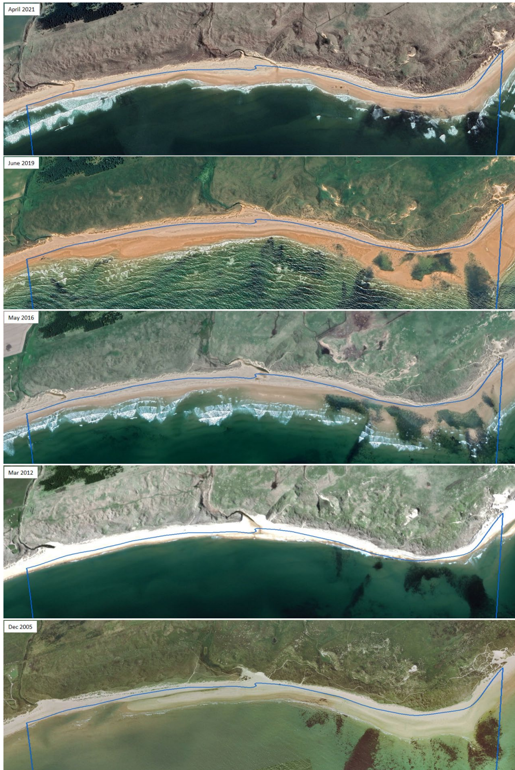
Figure 7-21 Morphological change at the landfall over the period 2005 to 2021 (Source: Google Earth)
