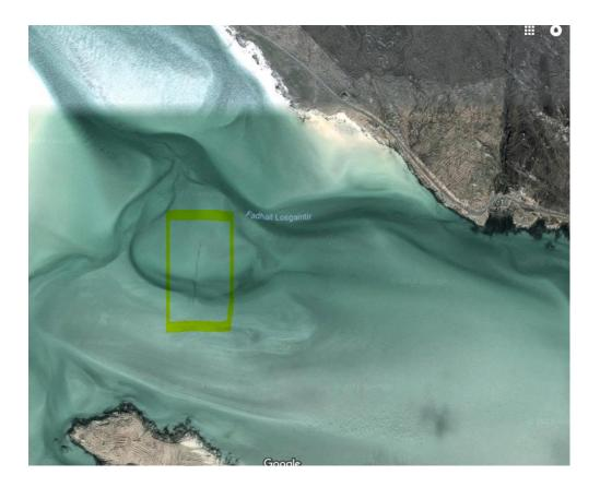
The solution we have allowed for includes weighting down the pipeline where the motion of the tidal stream has exposed the line.
