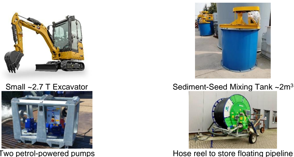
Figure 4: Envisioned equipment for the temporary works area
