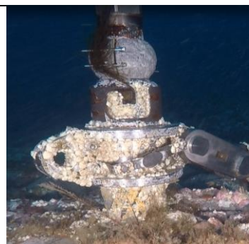
Fig 5 b) H-Link connection on Anchor 1
