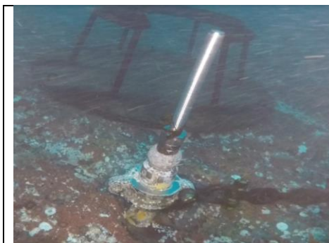
Fig 5 a) Anchor showing mooring chain with mooring line deployment frame in background.
