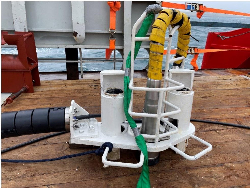
Figure 6 - HiCUP MkII Platform wet-mate connector frame
