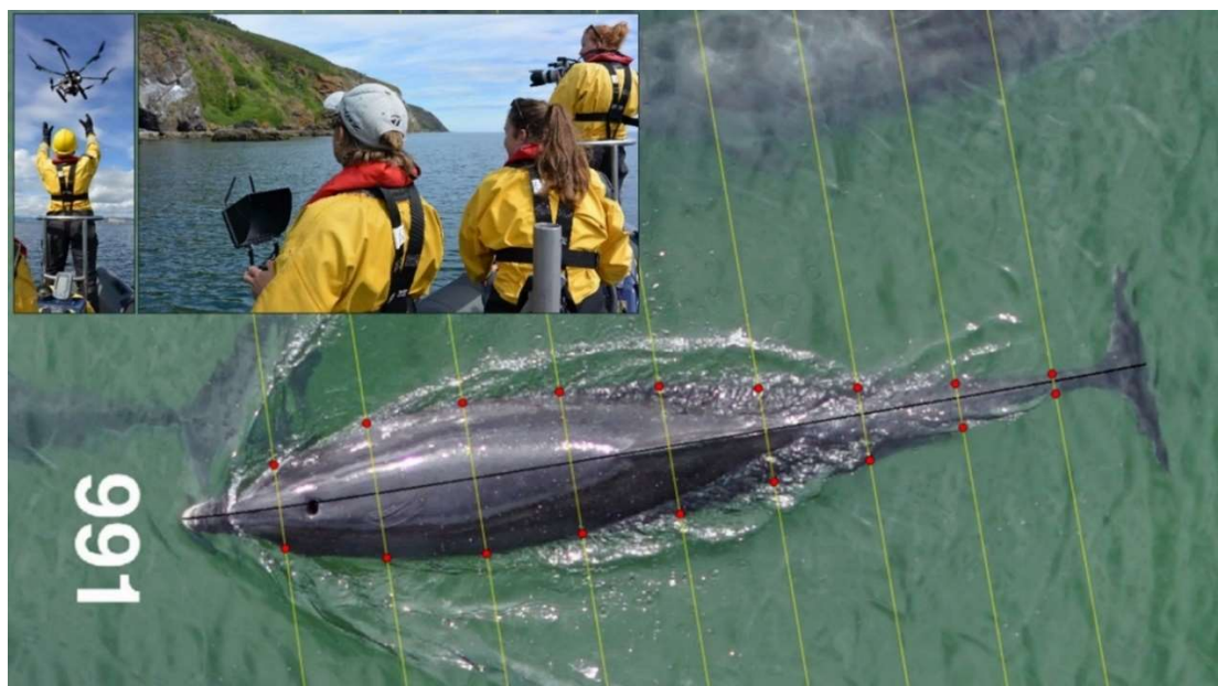
Figure 2. Picture illustrating UAV image of length and width measurements of a bottlenose dolphin, with inset photographs from a survey in the Moray Firth showing UAV launch and concurrent UAV and laser photogrammetry and photo-ID (Cheney et al submitted, Cheney et al 2017).
