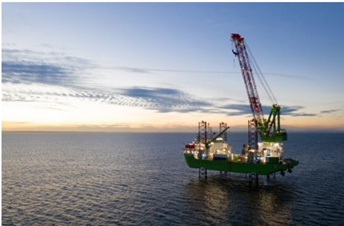
Figure 5-5: MV Apollo vessel for piling operations
