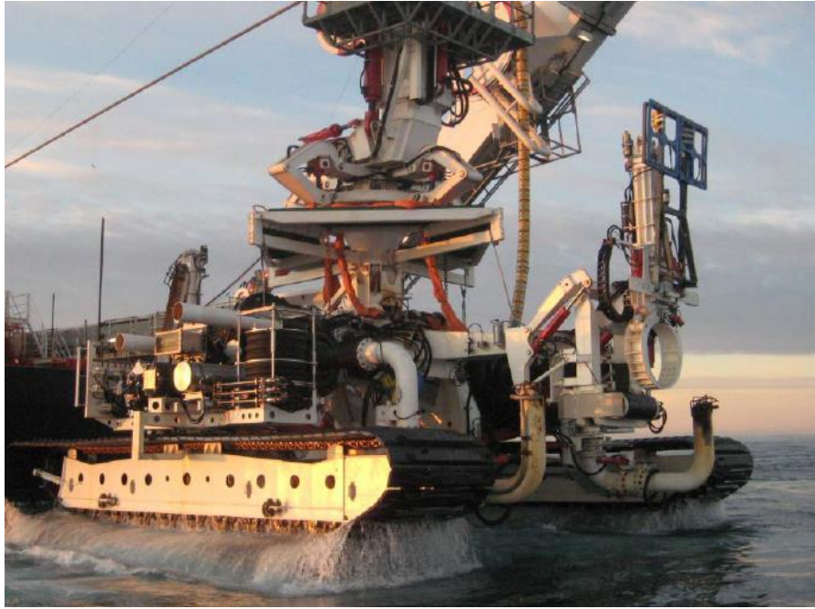
Figure 5-26: Typical cutting and jetting tracked burial tool
