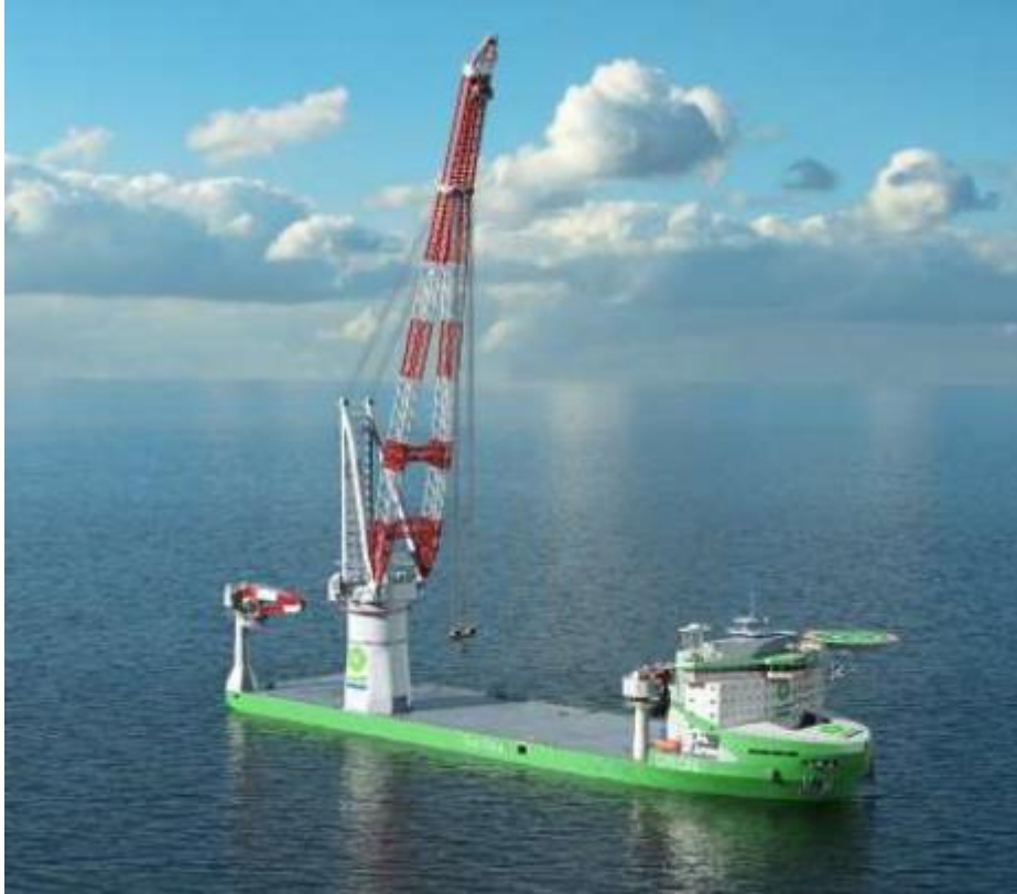
Figure 5-12: Indicative jacket installation vessel - HLV (e.g. Orion)
