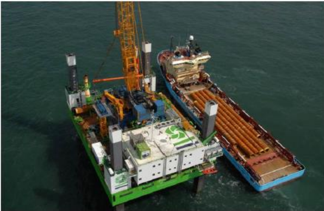
Figure 5-8: PSV Pile Delivery
