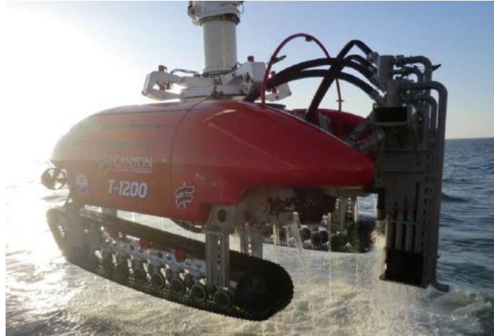
Figure 5-27: Typical jet trenching tool
