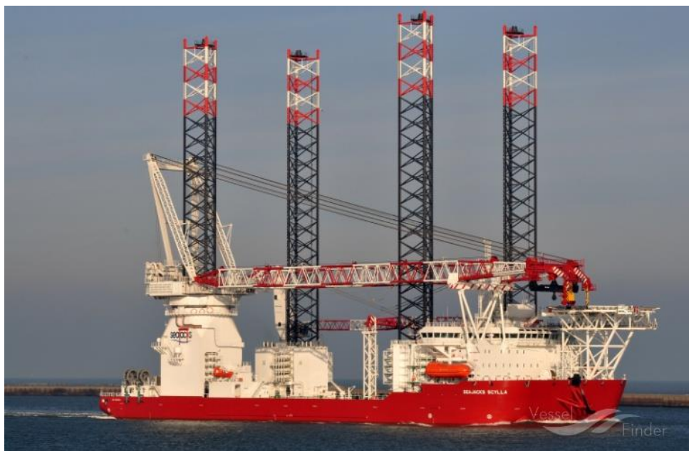
Figure 5-13: Indicative jacket installation vessel - JUV (e.g. Scylla)
