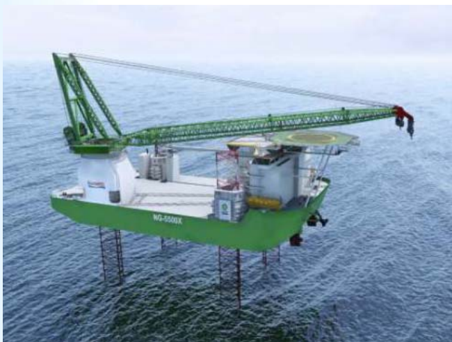
Figure 3-1: Typical jack-up vessel for piling operation
