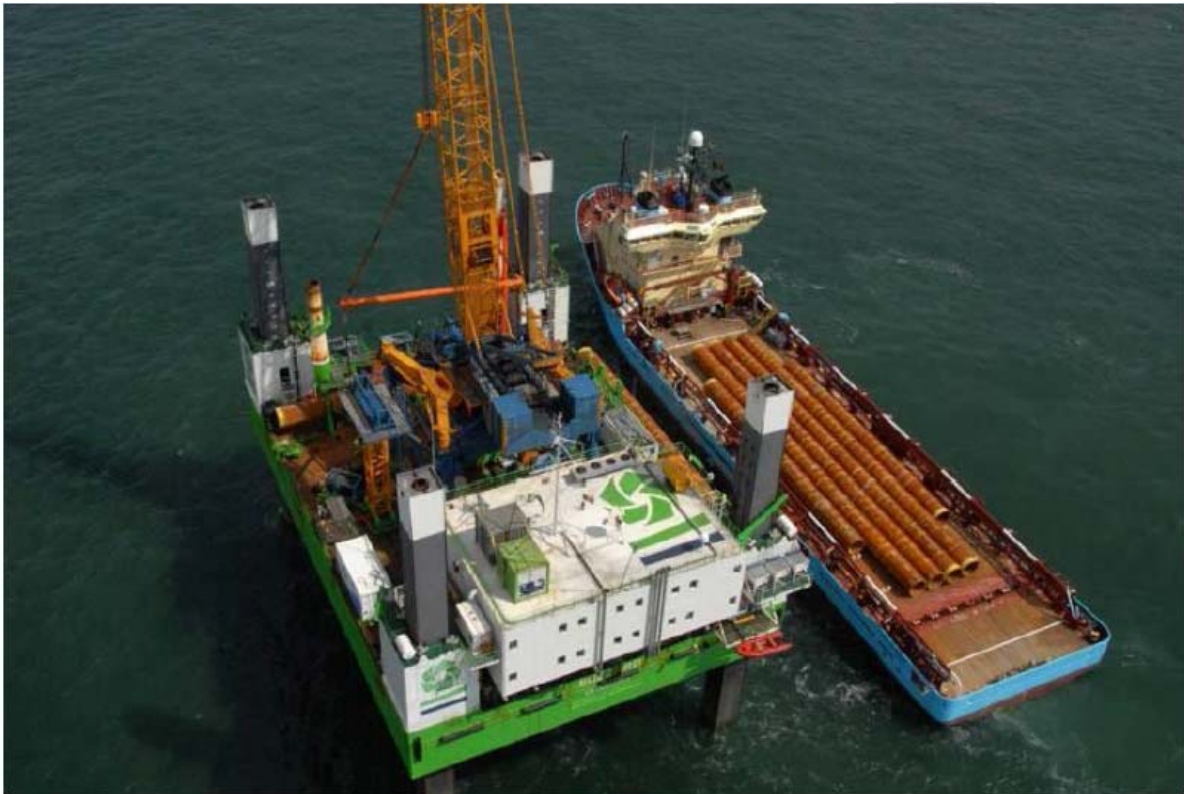
Figure 2: Example Jack Up Platform and Supply Vessel with pin piles
